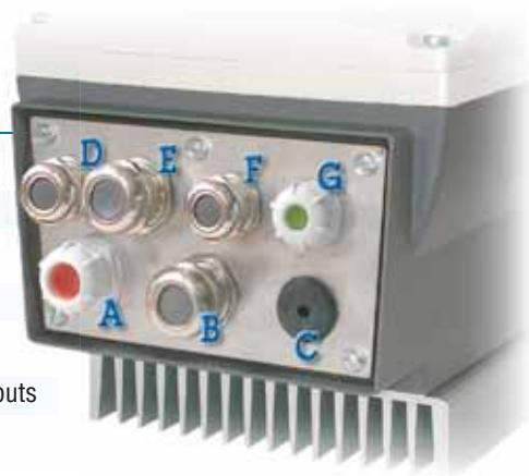
Note: The kit has 6 PE. The standard PE's are plastic, the EMC PE's are metal to ensure the continuity of the shielding and EMC conformity. If required by the number of cables, the hole "C" may be used with a plastic PE.
