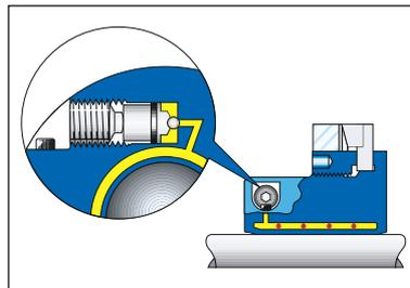
ETP-KN is designed acc. to the same principle as ETP-TECHNO but the expansion is only against the shaft. It is used for example for fastening of circular knives for slitting thin steel-plate when manufacturing beverage and food cans.
