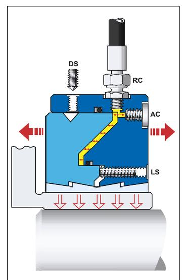
Mounting is done in a couple of minutes with hydraulic, even on large hollow shafts. Dismantling is as quick.
