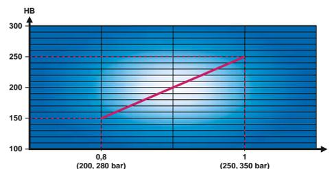
If the hardness of the hollow shaft is < 250 HB the surface might be damaged. This can be avoided by reducing the mounting pressure. The transmittable torque will then be proportionally reduced. For example a hardness of 150 HB, a reduction of the mounting pressure by 20% is recommended.
