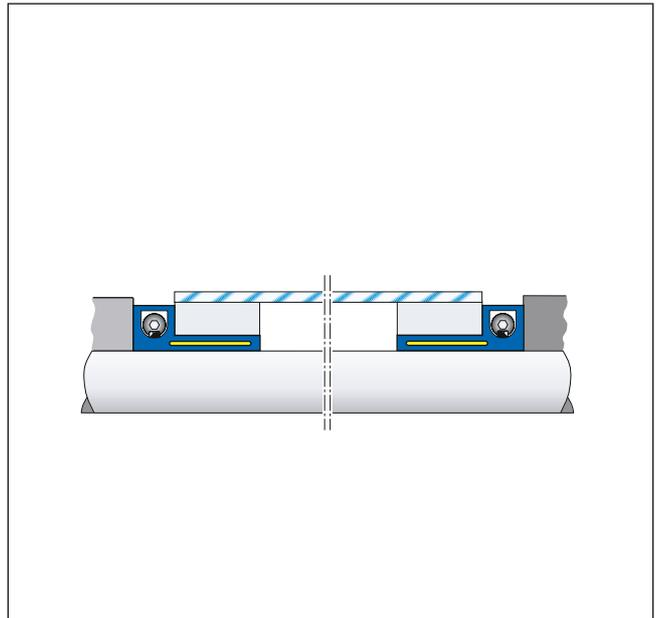
ETP-TECHNO gives advantages when being used to fasten printing cylinders in light materials for example aluminium. The cylinder can be changed 1000's of times, using the same ETP-TECHNO, with maintained good concentricity and repeatability. The radial access to the screw facilitates the handling and saves space.
