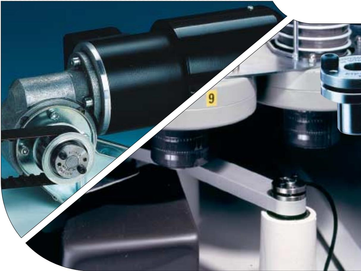
*ETP-MINI is far superior to keyways or setscrews because it allows an adjustable, backlash free joint. Typical applications are mounting of hubs on small electrical motors, steppermotors and encoders. As no keyways are needed, the shaft will not be weakened and the unbalance will be lower, which is very important at high speeds, as the motor bearing are sensitive to vibrations. Also available in stainless, ETP-MINI type R, suitable for the food processing industry etc.*
