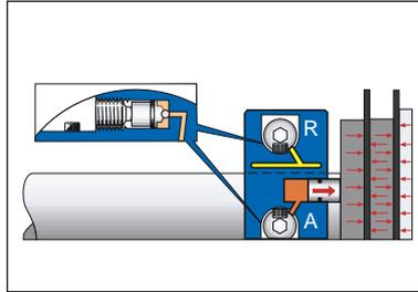
ETP-UNIGRIP has two separate hydraulic functions. When tightening the screw, R, ETP-UNIGRIP grips to the shaft. When tightening screw, A, 3 pistons are pressurized which creates a high axial force against the components which are going to be clamped.
