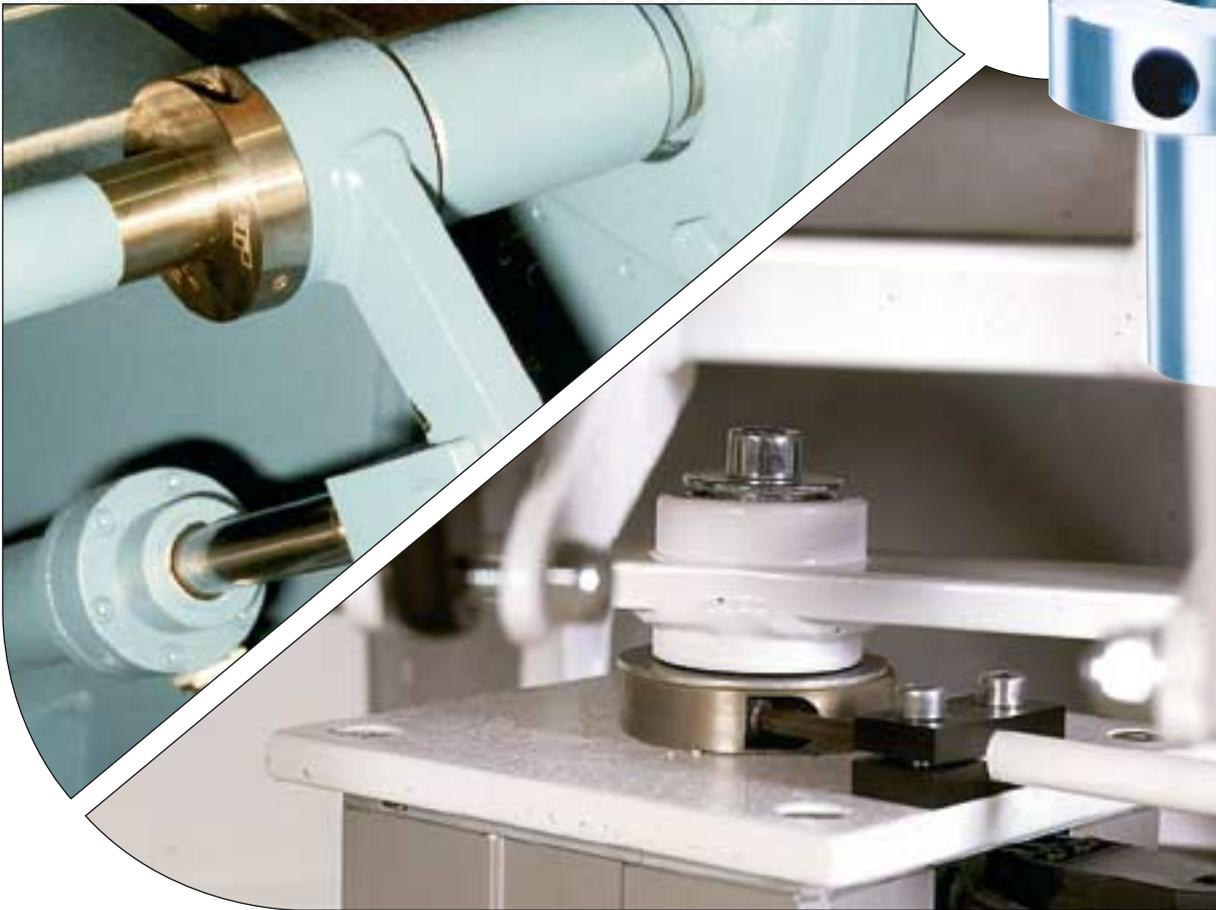
*ETP-EXPRESS has only one screw for pressurising, it is therefore specially designed for when there is a need for the repositioning of the hub to be done fast and accurately. The screw is tightened in the radial direction, this means that no space is used along the shaft for mounting tools. Other components can be mounted on the shaft all the way up to the flange. ETP-EXPRESS has extremely small built-in dimensions.*
