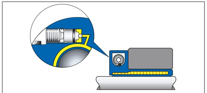
*When the pressure screw is tightened to the recommended tightening torque,  $T_t$ , the steel ball seals against the spherical seating. ETP-TECHNO will have created a uniform surface pressure against the shaft and hub.*
