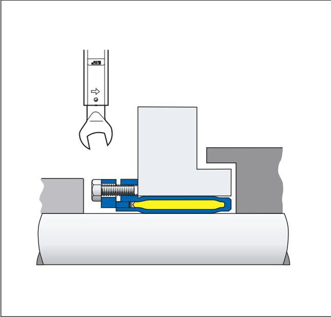
When designing in ETP-CLASSIC and the space is limited in the axial direction, hexhead screws can be used. They are available as accessories in quality 12.9 from us. As no dismantling screws are needed, ETP-CLASSIC can be easily dismantled. Stainless hex head screws, A4, are also available as accessories for ETP-MINI R.
