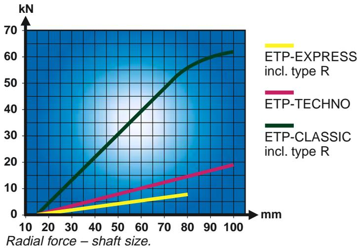
Most friction joints have a limited capacity to transmit radial forces and bending torque. Extreme levels of these loads can affect the function of the ETP connection. The values acc. to the diagram and table based on tests can serve as guide lines. ETP-MINI and ETP-HYLOC can transmit essentially higher radial forces than the other connections.
