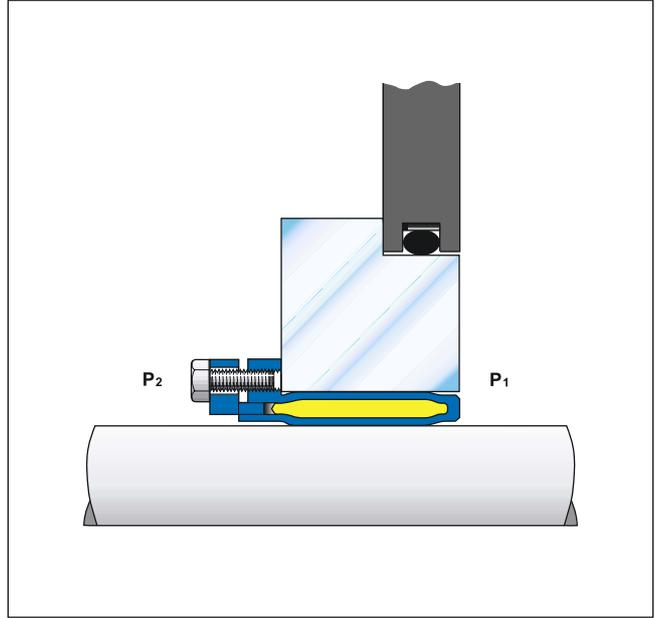
In humid environments, at varying temperature and with a hub made from aluminium ETP-CLASSIC type R can be used. Thanks to the flexibility of ETP-CLASSIC R at varied temperatures, it can be used in hubs of aluminium. Because of the even surface pressure and the lack of slotted sleeves, ETP-CLASSIC R can function as a sealing element up to a pressure difference,  $p_1 - p_2$ , of 50 bar.
