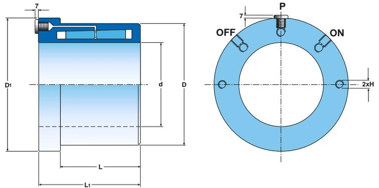
ETP-HYLOC is prepared for axial connection of the hoses (where the plastic plugs are situated). If radial connection is to be made, the steel plugs are moved to the axial connections and are tightened with a torque wrench to 20 Nm.
