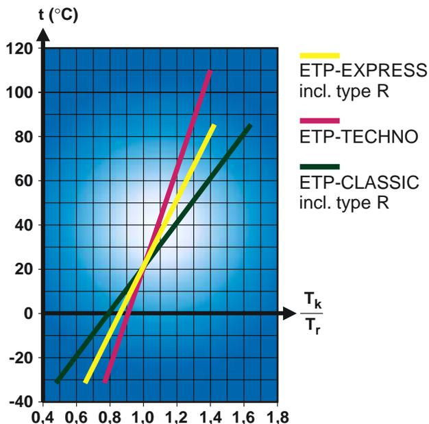
The pressure medium in the hydraulic ETP connections fills the double-walled steel sleeve and is effected by the differing volume expansion coefficient. This means that when the temperature rises, the pressure in the connection increases and a higher torque can be transmitted. The opposite is valid at decreasing temperature.
