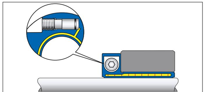
*When the pressure screw is tightened to the recommended tightening torque, the piston has reached the bottom of the bore. ETP-EXPRESS has created a uniform surface pressure against the shaft and hub.*
