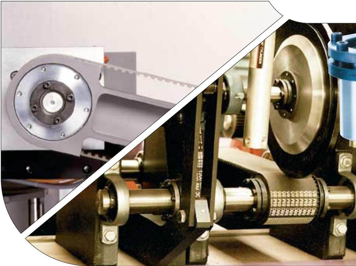
*ETP-CLASSIC is used in a large variety of applications, for mounting timing belt pulleys, camcurves and arms etc. Positioning along and between the shafts is easy and fast with a high precision. Service and maintenance are also quick because of the easy dismantling. ETP-CLASSIC is recommended for all normal needs.*
