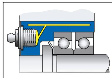
These ETP connections are designed to absorb the very small bearing play in a robot design. With the proper choice of tolerances and pressure in the connection the precision and repeatability of the robot has been improved.
