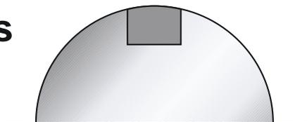
If there is a keyway in the shaft or hub, we recommend it to be filled in with for example some two component hardening medium (not for ETP-MINI or ETP-IMPRESS). The medium is then hand grind to the diameter of the shaft/hub. This prevents deformation and dismantling problems of the double-walled sleeve.
