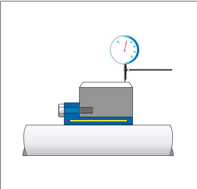
When manufacturing precision gears, they can be fastened with ETP- EXPRESS. If the gear is fixed in its position with an axial screw or pin before the last grinding operation, a repeatability within  $2 \mu\text{m}$  will be achieved.
