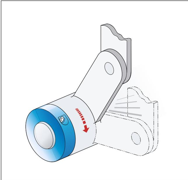
There is a linear ratio between the transmittable torque and the tightening torque for the screw for ETP-EXPRESS and ETP-TECHNO. The torque can be decided for when the connection slips by proper selection of hub/shaft tolerances and tightening torque. The connection can then be used as an overload protection with limited slipping.
