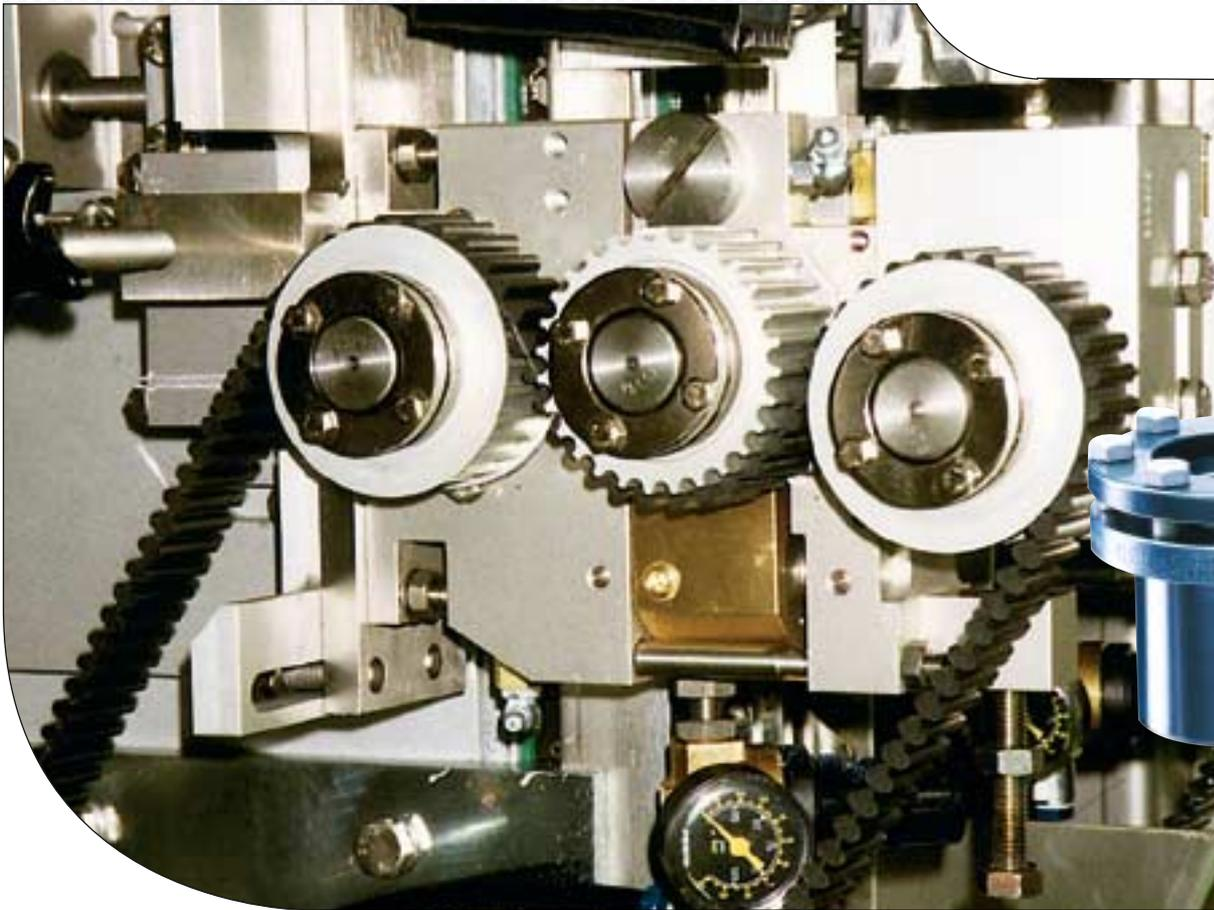
The demand from the food and process industries is increasing for stainless steel hub-shaft connections; surface coatings and plating are no longer sufficient. The most common sizes of ETP-CLASSIC are also available in stainless steel.
