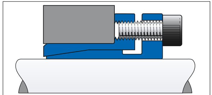
*The inner sleeve, for ETP-MINI incl. type R, has a light recess close to the flange in order to create a more uniform surface pressure to the shaft.*
