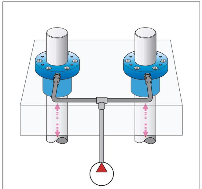
ETP-OCTOPUS is a connection where the pressure setting is done with an external pressure source. Suitable applications are when repositioning of parts are to be done frequently, fast and precise. Several connections can be clamped/loosened simultaneously. Separate brochure is available.
