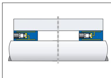
This ETP connection is used for fastening and centering a cylinder in a printing machine for beverage cans of aluminium. It has two separate pressure chambers, one for expansion to the shaft and one to the cylinder. The runout is better and the downtime shorter.
