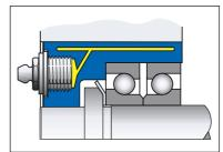
These ETP connections are designed to absorb the very small bearing play in a robot design. With the proper choice of tolerances and pressure in the connection the precision and repeatability of the robot has been improved.
