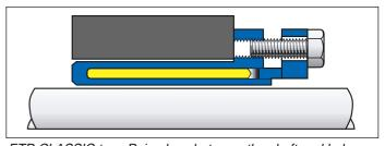
ETP-CLASSIC type R; in place between the shaft and hub ready for mounting.
