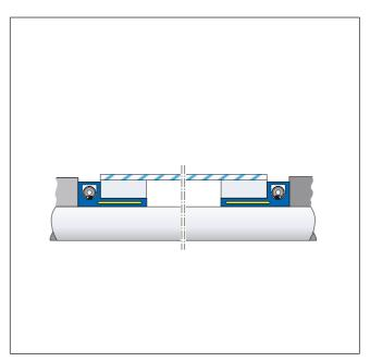
ETP-TECHNO gives advantages when being used to fasten printing cylinders in light materials for example aluminium. The cylinder can be changed 1000's of times, using the same ETP-TECHNO, with maintained good concentricity and repeatability. The radial access to the screw facilitates the handling and saves space.
