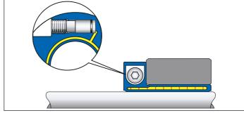
When the pressure screw is tightened to the recommended tightening torque, the piston has reached the bottom of the bore. ETP-EXPRESS has created a uniform surface pressure against the shaft and hub.
