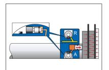
ETP-UNIGRIP has two separate hydraulic functions. When tightening the screw, R, ETP-UNIGRIP grips to the shaft. When tightening screw, A, 3 pistons are pressurized which creates a high axial force against the components which are going to be clamped.
