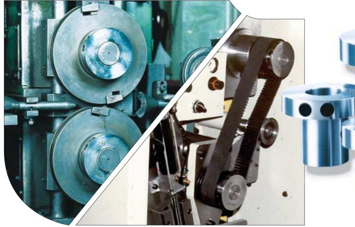
ETP-TECHNO is specially designed for applications where fast frequent changes or adjustments, with high precision are needed. ETP-TECHNO can be mounted/dismantled 1000's of times. It is very easy to mount ETP-TECHNO in a tight space, and it also has extremely good concentricity. ETP-TECHNO is the high precision joint among the ETP hub-shaft connections.
