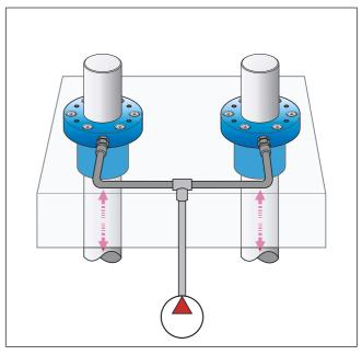
ETP-OCTOPUS is a connection where the pressure setting is done with an external pressure source. Suitable applications are when repositioning of parts are to be done frequently, fast and precise.
