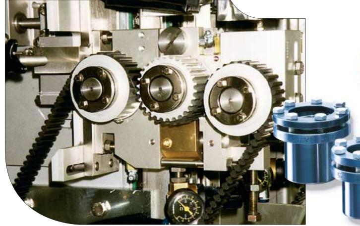
The demand from the food and process industries is increasing for stainless steel hub-shaft connections; surface coatings and plating are no longer sufficient. The most common sizes of ETP-CLASSIC are also available in stainless steel.
