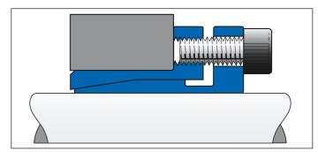
The inner sleeve, for ETP-MINI incl. type R, has a light recess close to the flange in order to create a more uniform surface pressure to the shaft.
