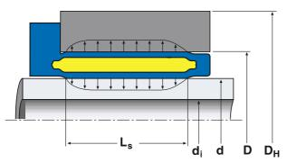
Built-in principle of ETP-connection.
