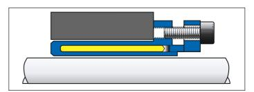
ETP-CLASSIC in place between the shaft and hub ready for mounting.
