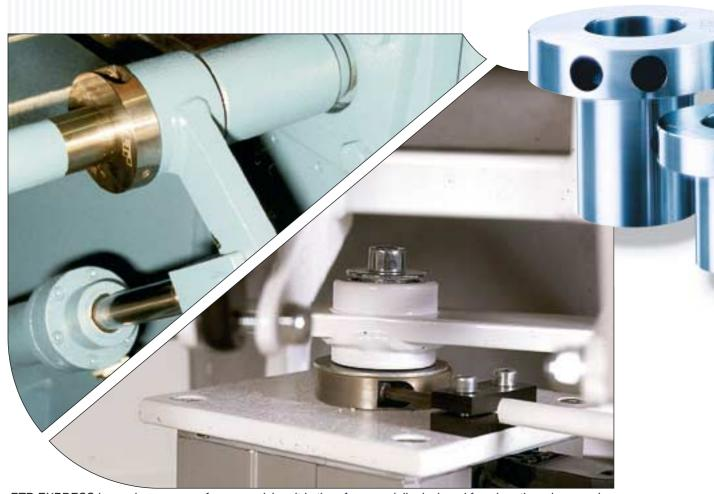
ETP-EXPRESS has only one screw for pressurising, it is therefore specially designed for when there is a need for the repositioning of the hub to be done fast and accurately. The scew is tightened in the radial direction, this means that no space is used along the shaft for mounting tools. Other components can be mounted on the shaft all the way up to the flange. ETP-EXPRESS has extremely small built-in dimensions.
