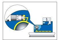
ETP-KN is designed acc. to the same principle as ETP-TECHNO but the expansion is only against the shaft. It is used for example for fastening of circular knives for slitting thin steel-plate when manufacturing beverage and food cans.
