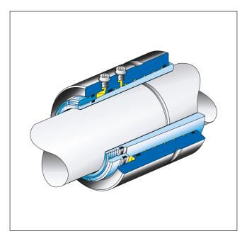
ETP-HYCON S is a hydro-mechanical shaft-shaft coupling for high torque and rigidity. The mounting is done, as for ETP-HYLOC, with an external pump. The design is type approved by for example DNV for use in the drive line for ships. Other important applications are in the steel-, paper-and other heavy industry where the requirements are for high torque, low weight, high rigidity and short down time. Separate brochure is available.
