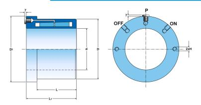
ETP-HYLOC is prepared for axial connection of the hoses (where the plastic plugs are situated). If radial connection is to be made, the steel plugs are moved to the axial connections and are tightened with a torque wrench to 20 Nm.
