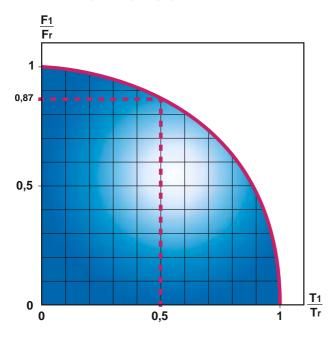
If axial force  $(F_1)$  and torque  $(T_1)$  are to be transmitted at the same time, the following formula is valid.
