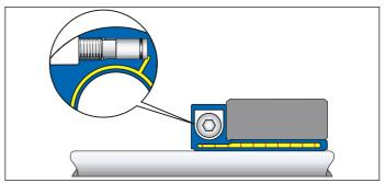
When the pressure screw is tightened to the recommended tightening torque, the piston has reached the bottom of the bore. ETP-EXPRESS type R will have created a uniform surface pressure against the shaft and hub.
