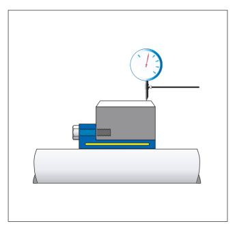
When manufacturing precision gears, they can be fastened with ETP- EXPRESS. If the gear is fixed in its position with an axial screw or pin before the last grinding operation, a repeatability within 2 µm will be achieved.
