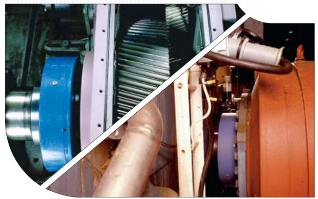
The connection of a hollow shaft, for example from a hydraulic motor or a gearbox, to a shaft is today often done with a mechanical shrink disc. These are built up of conical rings. When mounting a high radial force is needed to compress both the conical rings and the hollow shaft. This is achieved through a lot of screws with a high tightening torque. Mounting/dismantling causes long downtime which is expensive in the process industry for example in the pulp and paper industry.
