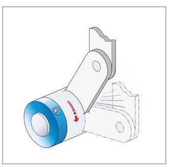
There is a linear ratio between the transmittable torque and the tightening torque for the screw for ETP-EXPRESS and ETP-TECHNO. The torque can be decided for when the connection slips by proper selection of hub/shaft tolerances and tightening torque. The connection can then be used as an overload protection with limited slipping.
