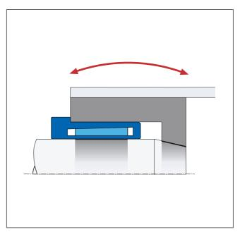
Long thin rollers subjected to high bending torque, can be fastened to stub shafts with ETP-HYLOC. To decrease the elastic deformation of the roller and make it easier to take up the bending torque, the inner part of the hub and the stub shaft can be designed with conical support surfaces. ETP-HYLOC gives good concentricity and fast changes.
