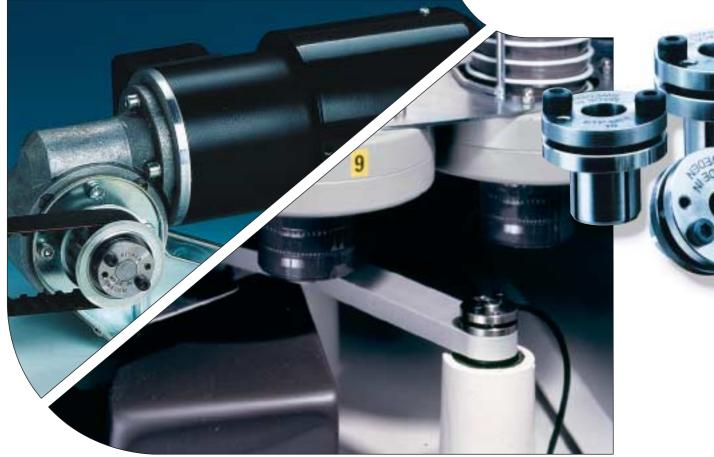
ETP-MINI is far superior to keyways or setscrews because it allows an adjustable, backlash free joint. Typical applications are mounting of hubs on small electrical motors, stepmotors and encoders. As no keyways are needed, the shaft will not be weakened and the unbalance will be lower, which is very important at high speeds, as the motor bearing are sensitive to vibrations. Also available in stainless, ETP-MINI type R, suitable for the food processing industry etc.
