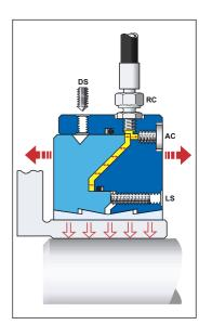
Mounting is done in a couple of minutes with hydraulic, even on large hollow shafts. Dismantling is as quick.
