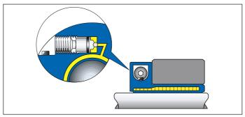
When the pressure screw is tightened to the recommended tightening torque, Tt, the steel ball seals against the spherical seating. ETP-TECHNO will have created a uniform surface pressure against the shaft and hub.
