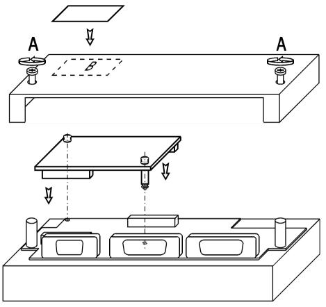
Figure 22- Mounting the communication modules
