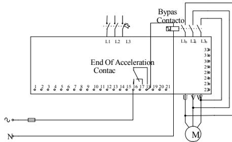
End of Acceleration contact is activated after an adjustable time delays “Run Contact Delay” – see page 29 at the end of start-up period, closing the by-pass contactor.
