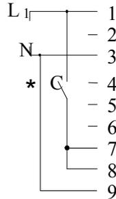
8. External Fault contact. The starter will trip 2 sec after C closes.
