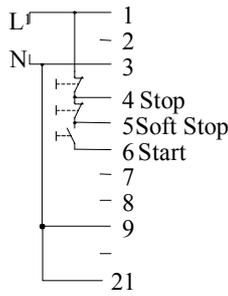
2. Start-Stop push buttons, Separate sources for Control Supply and Control Inputs. If Soft Stop is not used, connect a jumper between terminals 4-5.
