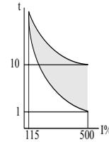
Adjustable between 75-150% of motor's FLA and factory set at 115%.
