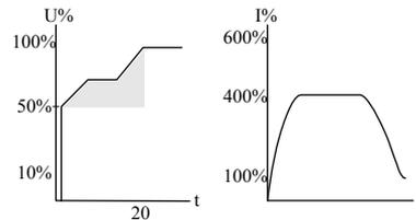
Voltage and current increase until current reaches “Current Limit value”. The voltage is held at this value until motor is close to nominal speed, then current will begin to decrease. The RVS-DN continues to ramp-up the voltage until reaching nominal. Motor speed smoothly accelerates to full speed.
