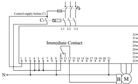
Upon starting, the “Immediate” contact is activated releasing the brake and allowing the voltage to ramp up (this contact will operate without a delay as long as “Immediate Relay ON delay” is set to 0 – see page 27). Upon stopping, the contact returns to its original position and the brake will close.
