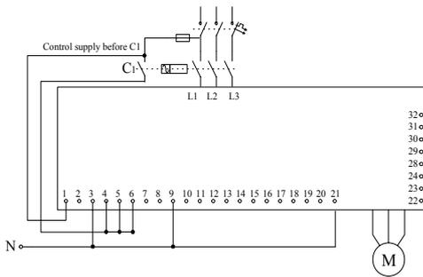
This system is mainly used when the RVS-DN is retrofitted into an existing system, to reduce modifications in existing installations.
