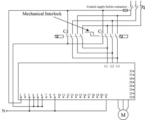
The start-stop control is by a N.O auxiliary contact in each of the two series contactors  $C_1$  &  $C_2$ . Closure of either contactor will supply main power and a start signal to the RVS-DN.
