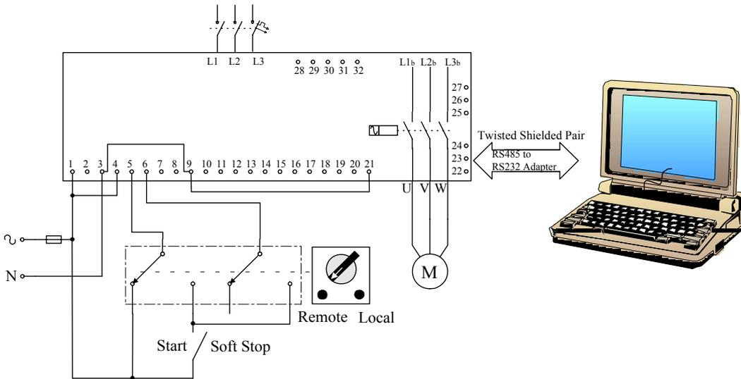
The communication enables remote parameter settings and reading. For start, stop, soft-stop, dual adjusts, etc terminals 4 and 5 must be wired as shown.
