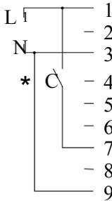
7. Close C to operate Dual Adjust. Slow Speed Reversing or Reset – as selected.
