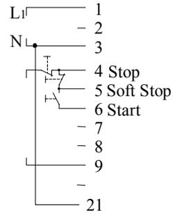
3. Motor will soft start when C closes and stops immediately when C opens.
