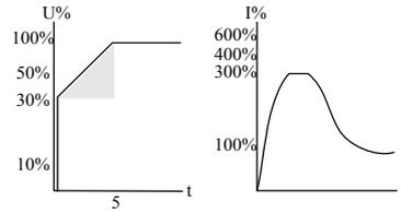
Voltage quickly increases to the Initial Voltage value and then gradually ramps-up to nominal. Current simultaneously and smoothly increases to reach Current Limit setting or less, before smoothly decreasing to the operating current. Motor speed will accelerate to full speed quickly and smoothly.
