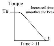
**Note:** Always use Stop Curve 0. If motor stalls quickly instead of slowly decreasing its speed, select Stop Curve 1, 2, 3 or 4 if necessary.
