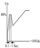
After this pulse, the voltage is ramped down to Initial Voltage setting, before ramping up again to full voltage according to Start Parameters settings.
