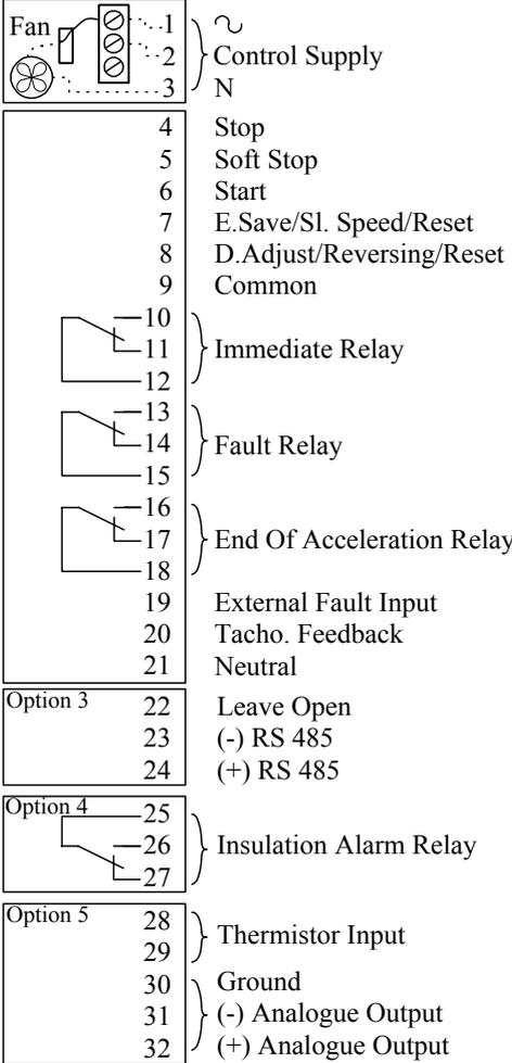
Fusing – Control Supply must be protected by a 6A fuse. It is recommended to use a separate fuse for the auxiliary circuits.
