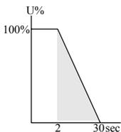
Used for controlled deceleration of high friction loads. Determines motor's voltage ramp down time. Range: 1-30 sec. (consult factory for extended range).
