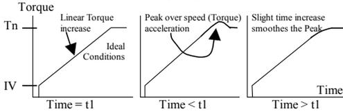
**Note:** Always starts with Start Curve 0. If towards end of acceleration, peak torque is too high (pressure is too high), proceed to Curve 1, 2, 3 or 4 if necessary.
