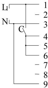
4. Motors will soft start when C closes and soft stop when C opens
