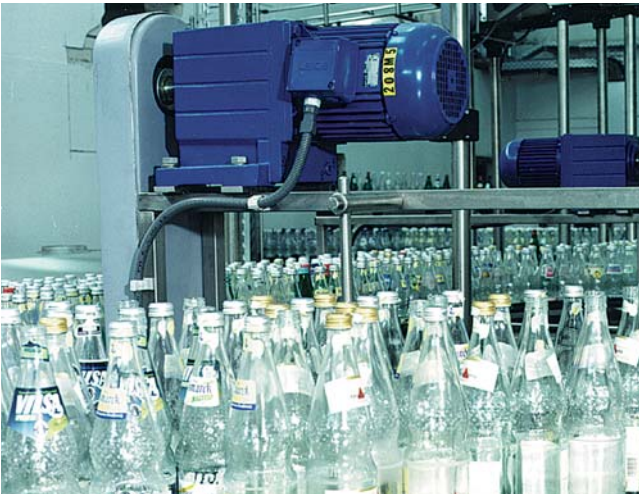
G-Motion drives conveyors in bottling plant
