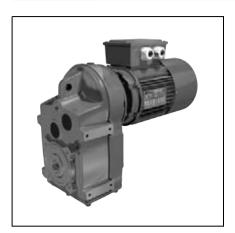
Manubloc 3000 geared motors with parallel gears are used to adapt the speed of the electric motor to that of the driven machine. Their size is therefore determined by the motor power (P) expressed in kilowatts (kW) and the output rotation speed of the gearbox  $(_nS)$  in revolutions per minute  $(min^{-1})$ . The main characteristic of the speed reducer is the rated output torque  $(M_{nS})$  expressed in Newton-metres (N.m):
