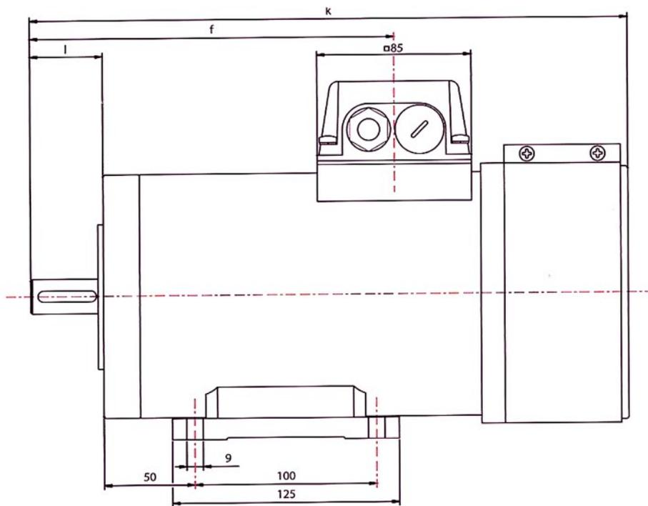
Extended shaft on non-drive end is an optional extra for fitting of tacho or brake.
