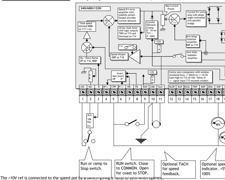
Note. The AVF/tach select switch must be set, and the appropriate speed scale range selected for the max feedback volts, depending on the source of speed feedback.
