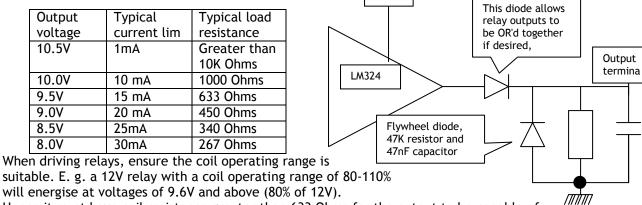
will energise at voltages of 9.6V and above (80% of 12V). Hence it must have coil resistance greater than 633 Ohms for the output to be capable of
