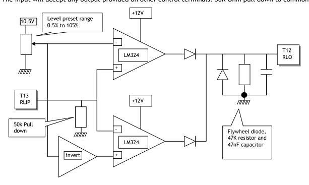
OVLD. Overload. This output goes high (+10.5V) if the current demand exceeds 100% and the stall timer starts timing. Flywheel diode to COM. See T12 RLOP for details of the output drive capability and configuration.
