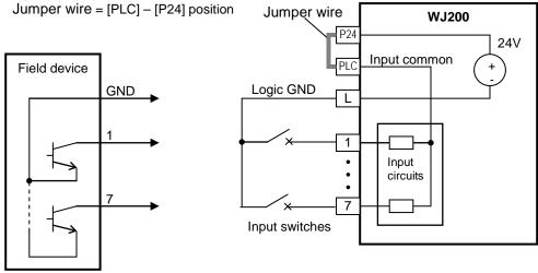
Open collector outputs, NPN transistors
