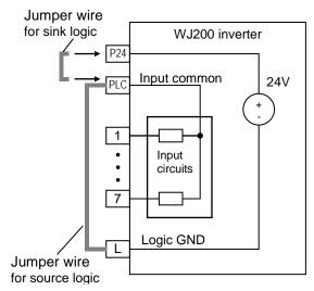
The wiring diagram on the following pages show the four combinations of using sourcing or sinking inputs, and using the internal or an external DC supply.
