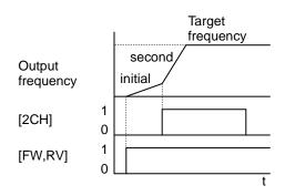
In the graph shown above, the [2CH] becomes active during the initial acceleration. This causes the inverter to switch from using acceleration 1 ( $\Phi$ 002) to acceleration 2 ( $\Delta$ 092).
