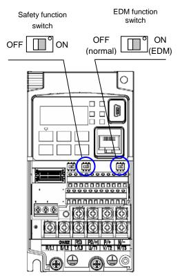
please turn the EDM function switch on. EDM output is automatically assigned on intelligent output terminal 11.
