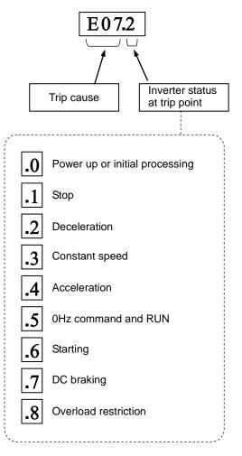
Note: Indicated inverter status could be different from actual inverter behavior. e.g. When PID operation or frequency given by analog signal, although it seems constant speed, acceleration and deceleration could be repeated in very short cycle.
