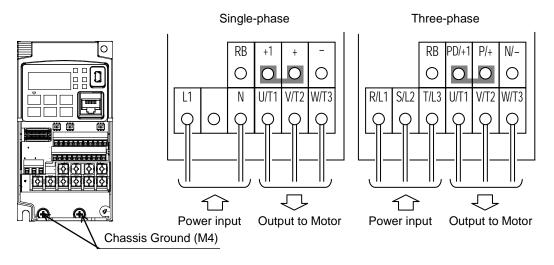
Single-phase 200V 0.75 to 2.2kW Three-phase 200V 1.5, 2.2kW Three-phase 400V 0.4 to 3.0kW
