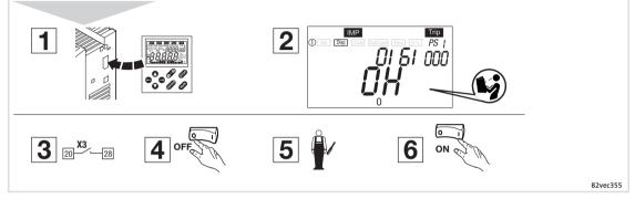
Reset the drive controller in this way if a fault occurs (TRIP reset):
