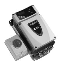
The PX-Disconnect option is an IP66/Nema 4X 3-pole padlockable 16A switch, with NO-NC auxiliary contacts. PX-Disconnect is supplied fitted on a plate ready to be fixed on the side of the drive.
