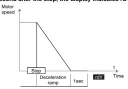
**rP.dC:** Stop on deceleration ramp with DC injection for an imposed period of time.
