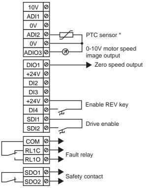
In this configuration, Run/Stop commands and the speed reference come from the keypad.
