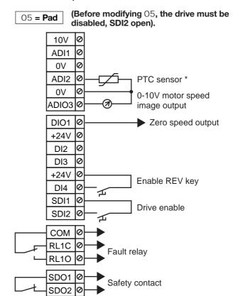
\* If the motor does not have a thermal sensor, place a shunt between terminals ADI2 and the 0V.
