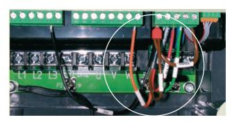
The PX-Brake Contactor Secure option includes the brake control PX-Brake Contactor option and the PX-Secure option for the secure disable input function on the same card. For information on these options, refer to sections 6.1.4 and 6.1.5.
