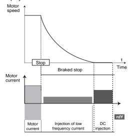
dC-t ( ): Stop on DC injection with an imposed period of time.
