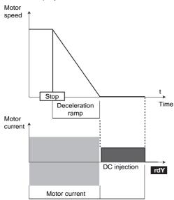
**dC-O** (**1**): Stop by DC injection braking, and elimination at zero speed.
