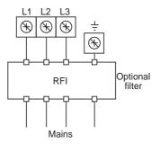
The filter is connected to the mains supply, without any special tools, on an IP66/Nema 4X dust and damp proof insulation displacement connector.
